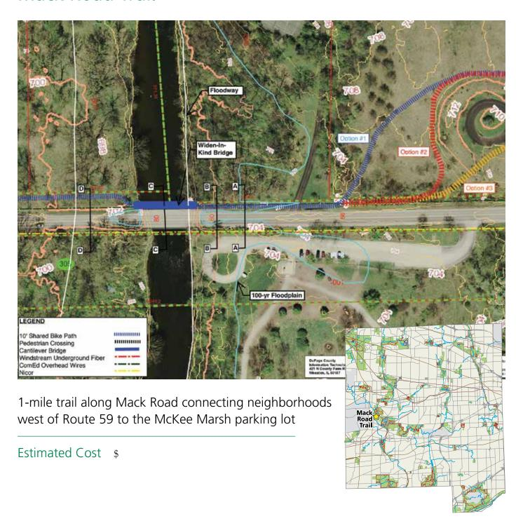
The project will construct a 1-mile-long, 10-foot-wide multipurpose asphalt path within the right-of-way on the north side of Mack Road between Route 59 and the turnaround at the McKee Marsh parking lot. It will also modify the pedestrian signal at Route 59 to connect the trail to sidewalks and trails within the Fox Hollow subdivision. Warrenville will expand and upgrade the bridge on Mack Road to accommodate an elevated path.
