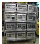
Rolling bank of small stainless-steel animal cages (9 cages), cages are removable; dimensions of unit 80" high x 65" wide x 26" deep.
